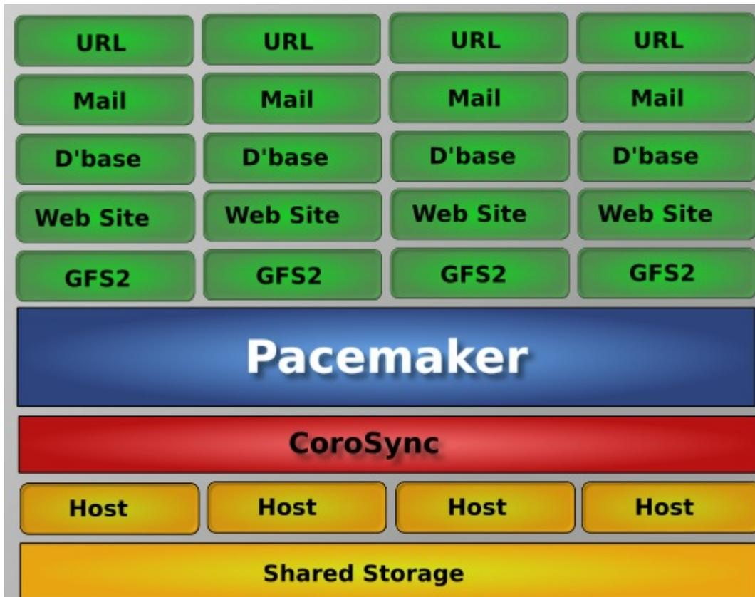
ACTIVE / ACTIVE ( N TO N REDUNDANCY )
